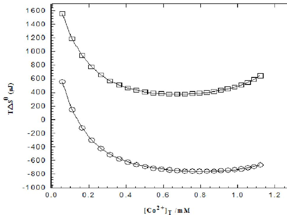
**Figure 3.** Comparison between the experimental entropies at 300 K (O) and 310 K (□) for  $\text{Co}^{2+}$ +CALI interactions in and calculated data (lines) via equations 7 and 8.
