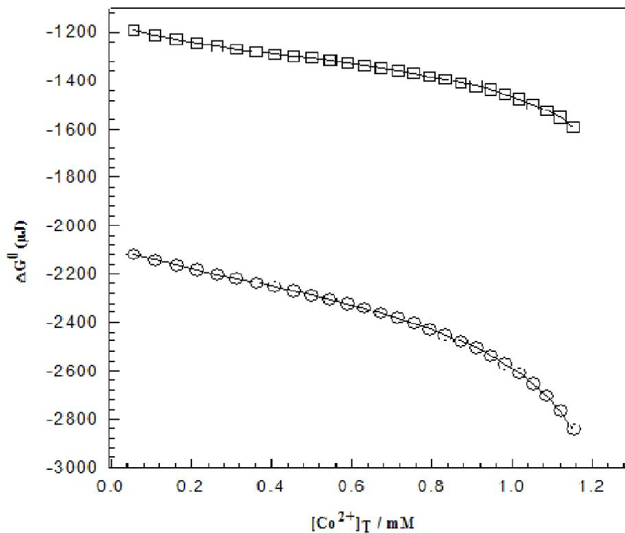
**Figure 2.** Comparison between the experimental Gibbs free energies at 300 K (O) and 310 K (□) for  $\text{Co}^{2+}$ +CALI interactions in and calculated data (lines) via Equations 7 and 8.
