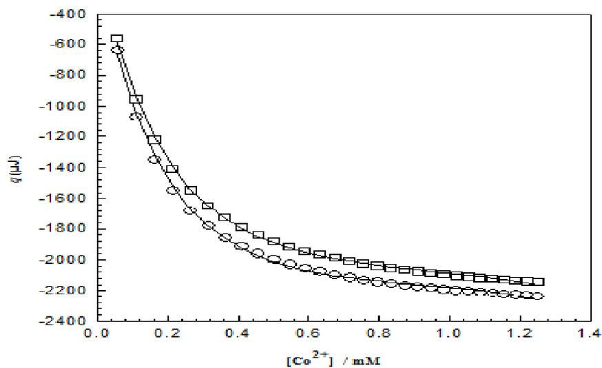
**Figure 1.** Comparison between the experimental heats for  $\text{Co}^{2+}$ +CAII interactions at 300 K (O) and 310 K ( $\Upsilon$ ) and calculated data (lines) via Equation 1.
