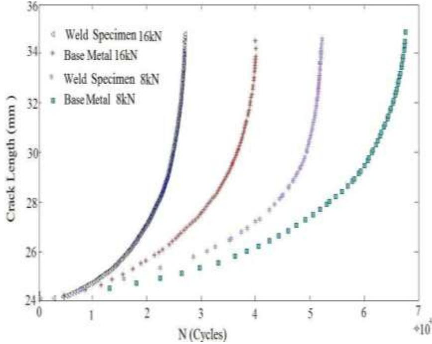
Figure 3. Crack length vs. Number of cycles.
