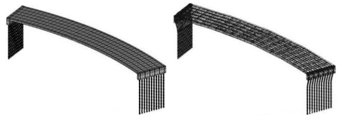
Figure 4. Undeformed and deformed shape of a curved integral abutment bridge with 400 ft radius and 4 to 50 ft spans with 28.65° of curvature with piles in very stiff clay soil profile with 9 ft deep predrilled holes filled with loose sand. The bridge is subjected to a thermal load of \Delta T_{\text{slab}} of 120° F and \Delta T_{\text{the rest}} of 90° F. A deflection scale factor of 40 is used to enlarge the displacement of the bridge structure.
