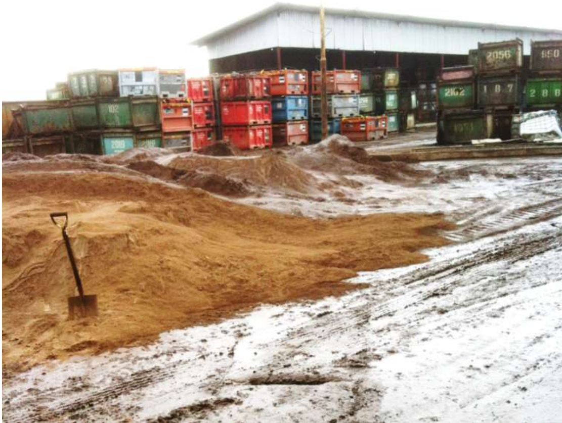
Figure 4. Heap of pre-treated drill cuttings from the anaerobic thermal desorption unit (ATDU) of a commercial treatment facility in the Niger Delta, Nigeria.
