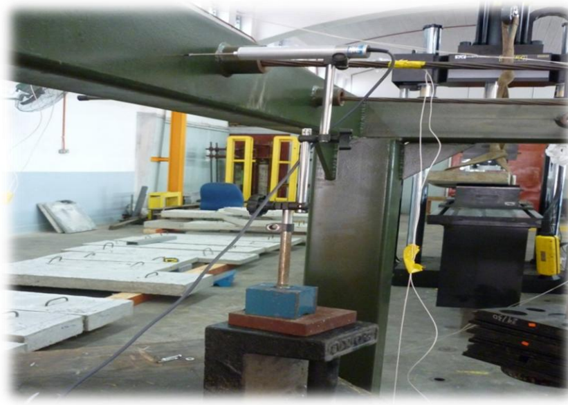
Figure 5. Linear variable differential transformer used on steel frame.
