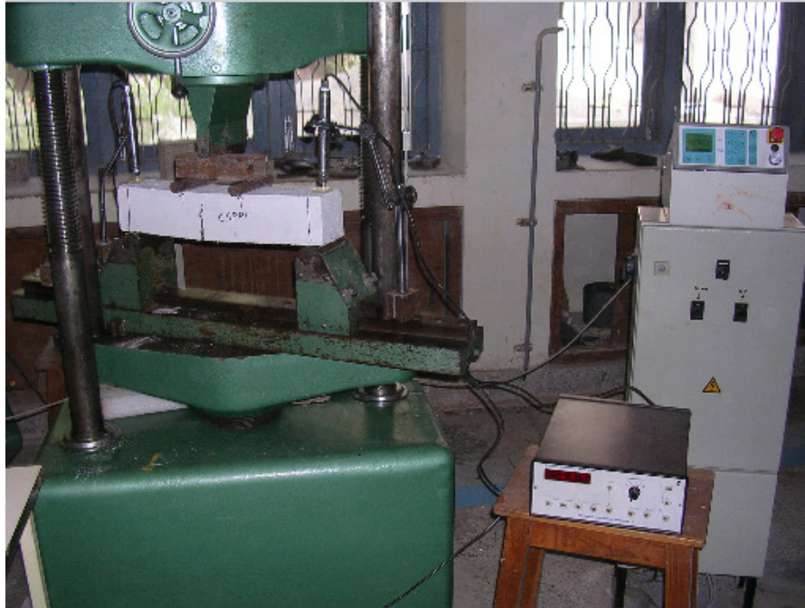
Figure 1. Experimental setup of flexural test.
