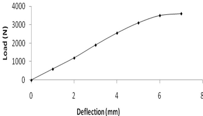
**Figure 2.** Load-Deflection Relation for the Nigerian Ekki in bending parallel to the grain.
