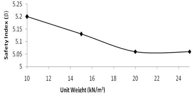
**Figure 6.** Safety Index - Unit Weight Relation for the Nigerian Ekki bridge beam in bending parallel to the grain.
