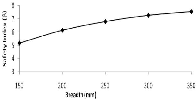
**Figure 5.** Safety Index - Breadth Relation for the Nigerian Ekki bridge beam in bending parallel to the grain.
