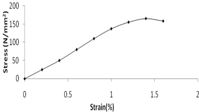
**Figure 1.** Stress-Strain Relation for the Nigerian Ekki timber in bending parallel to the grain.
