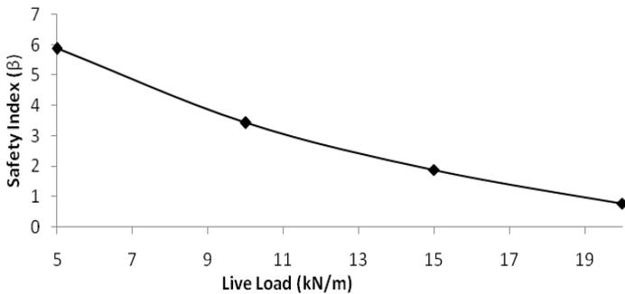
**Figure 4.** Safety Index - Live Load Relation for the Nigerian Ekki bridge beam in bending parallel to the grain.
