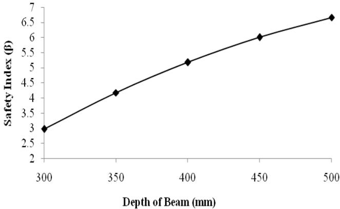
**Figure 3.** Safety Index - Depth Relation for the Nigerian Ekki bridge beam in bending parallel to the grain.
