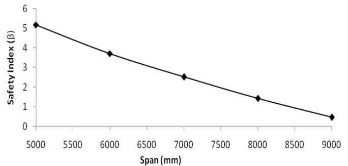
**Figure 7.** Safety Index - Span Relation for the Nigerian Ekki bridge beam in bending parallel to the grain.
