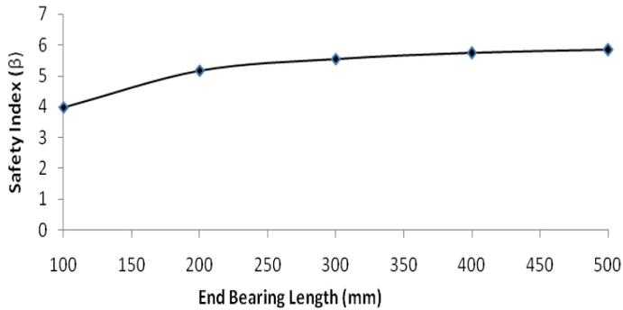
**Figure 8.** Safety Index - End Bearing Length Relation for the Nigerian Ekki bridge beam in bending parallel to the grain.
