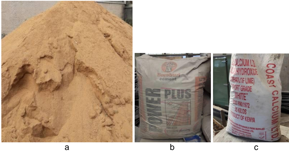
Figure 2. Materials for brick manufacture: (a) river sand, (b) ordinary portland cement, and (c) hydrated lime.
