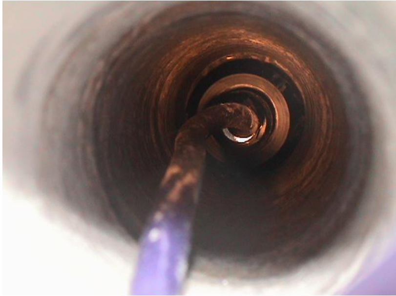
Figure 8. VW biaxial stressmeter position in the drill hole.
