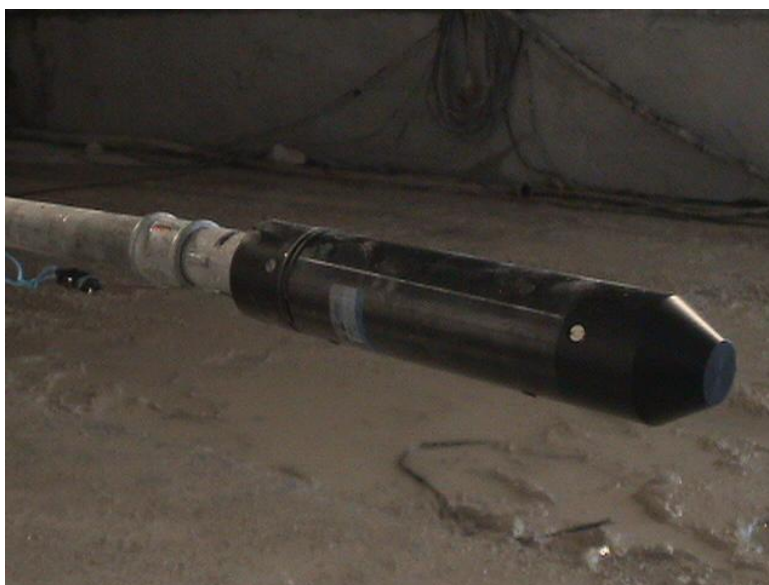
Figure 7. VW biaxial stressmeter.
