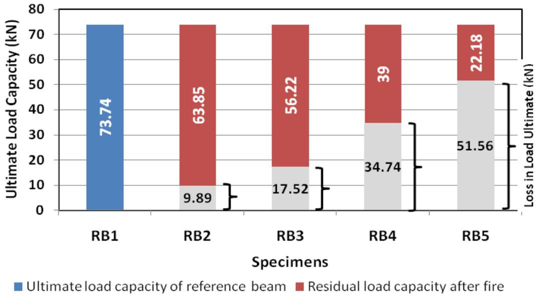
Figure 9. Ultimate load capacities of RC rigid beams.
