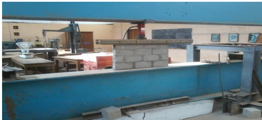
Figure 3. Test Set-up for masonry wallets compressive strength.
