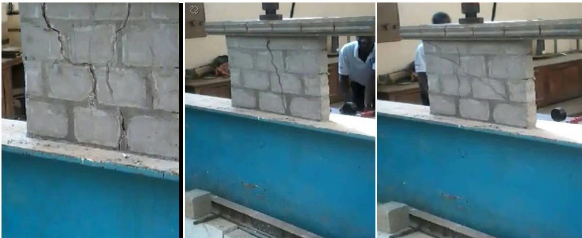
Figure 8. Crack patterns of failed wallets.
