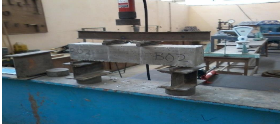
Figure 1. Set up for flexural tensile strength test.
