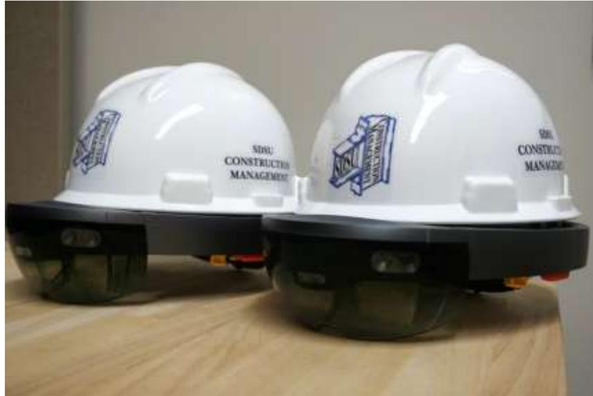
**Figure 2.** Two HoloLens with Trimble hard hat solution used in this study.
