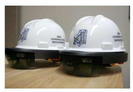
Figure 2. Two HoloLens with Trimble hard hat solution used in this study.
