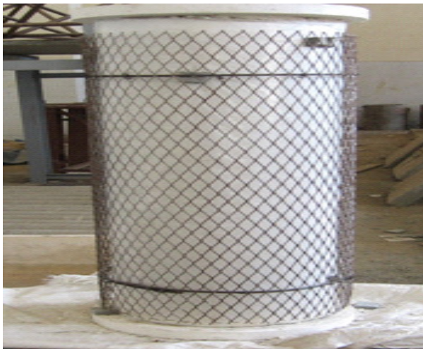
Figure 5. Steel in the form.
