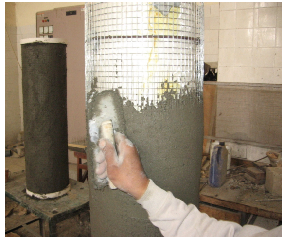
Figure 6. Casting the pipe by plastering.
