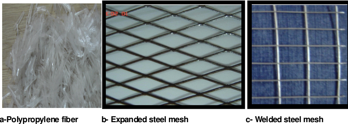
Figure 1. Reinforcement steel meshes and fibers used.
