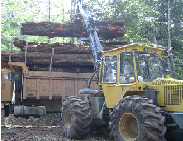
Figure 1. Loading operation by HSM 904 skidder in Dales Kheil forest (Rafiei et al., 2009).
