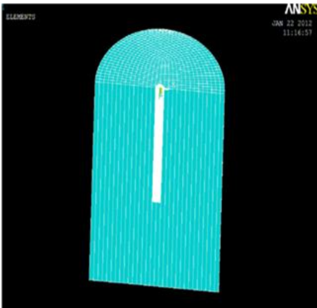
Figure 12. The meshing of the pile and soil.
