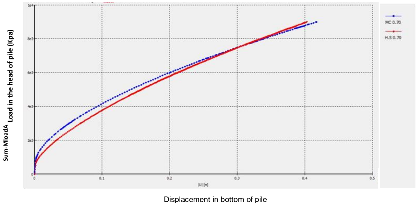
Graph 1. The settlement of pile for the interface coefficient of 0.70 (Mc and Hs).
