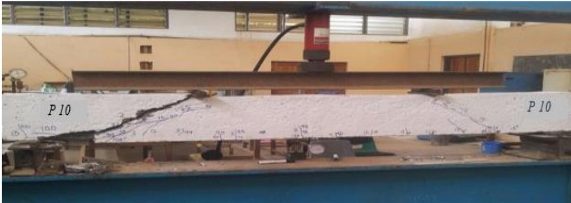
Figure 2. Test set up, instrumentation and failure mode.
