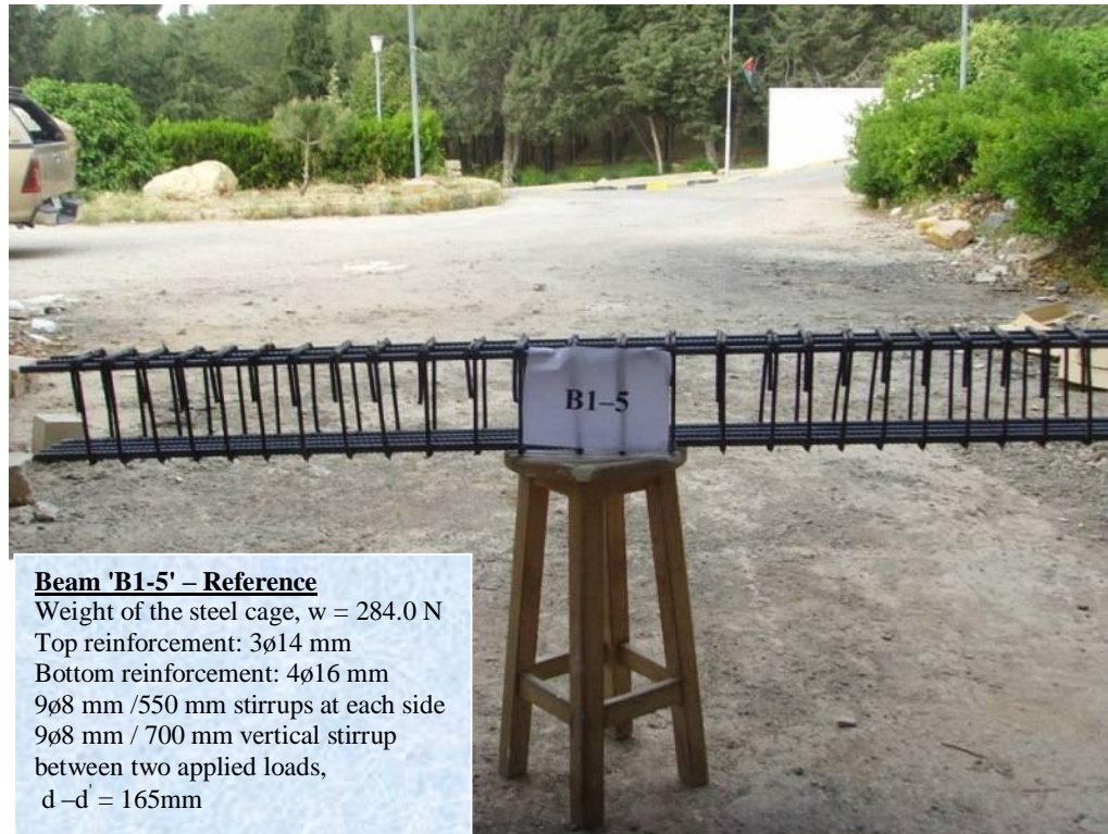
Figure 4. Steel cage for beam B1-5.
