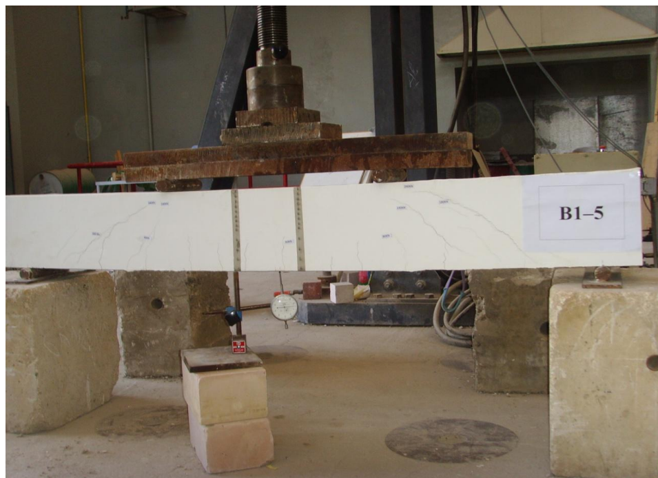
Figure 10. Mode of failure of the reference beam, B1-5.
