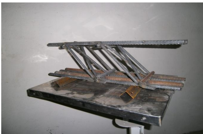
Figure 3. Rectangular swimmer bar system with cross bracings.
