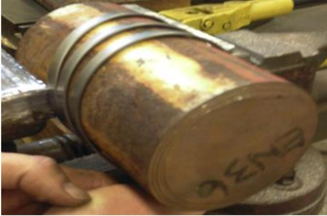
**Figure 2.** Experimental simulation of reverse bending of tensile armour wire.
