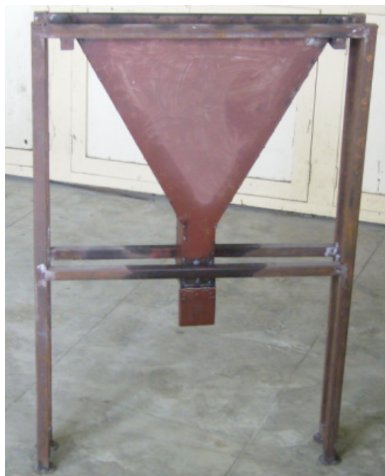
Figure 6. V- Funnel test apparatus.
