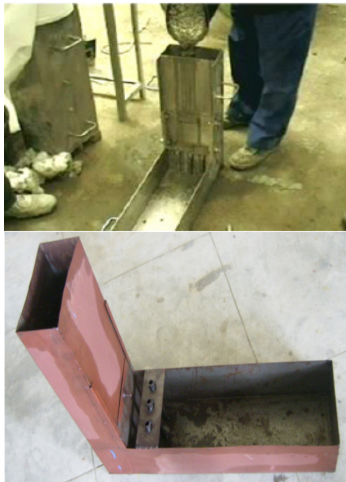
Figure 7. L-Box test apparatus.
