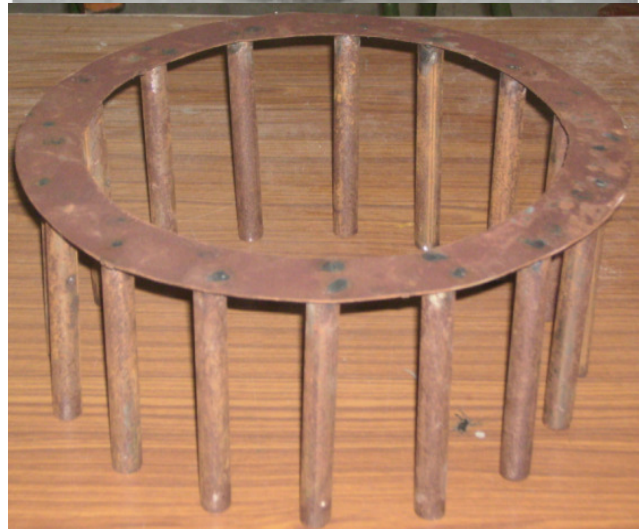
Figure 5. J-Ring test apparatus.
