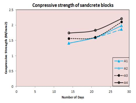
**Figure 1.** A graph of compressive strength of sandcrete blocks. A1-Curve for sandcrete blocks containing 0% coarse aggregate; A2-Curve for sandcrete blocks containing 5% coarse aggregates; A3-Curve for sandcrete blocks containing 10% coarse aggregates; A4--Curve for sandcrete blocks containing 15% coarse aggregates.
