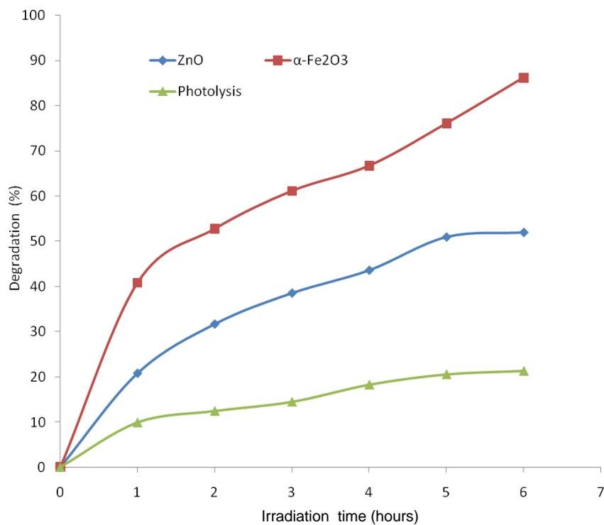
**Figure 4.** Effect of irradiation time on the photolytic and photocatalytic degradation of phenol using ZnO and  $\alpha$ -Fe<sub>2</sub>O<sub>3</sub>.
