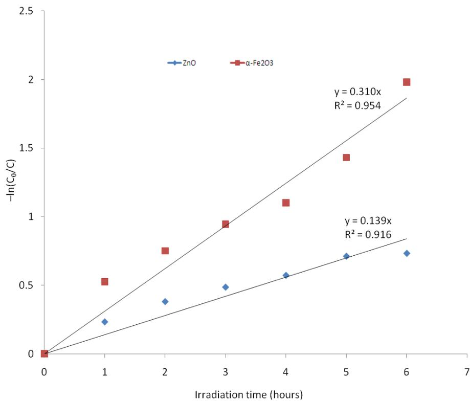
**Figure 5.** Pseudo first order kinetic plot for the photocatalytic degradation of phenol using ZnO and  $\alpha$ -Fe<sub>2</sub>O<sub>3</sub>.
