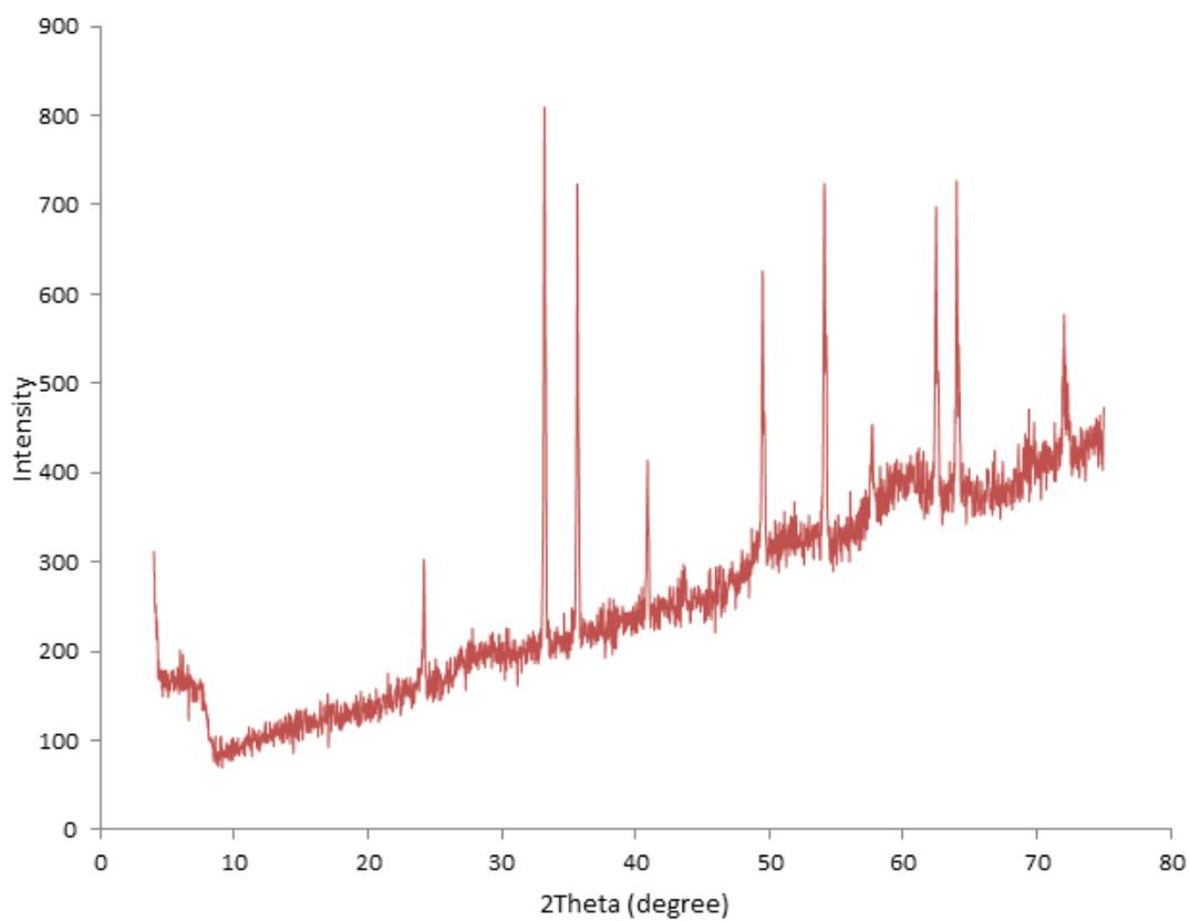
**Figure 2.** XRD pattern of the synthesized  $\alpha$ -Fe<sub>2</sub>O<sub>3</sub>.
