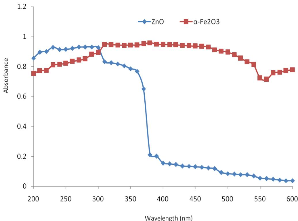
**Figure 3.** UV-Vis absorption spectra of the synthesized ZnO and  $\alpha\text{-Fe}_2\text{O}_3$ .
