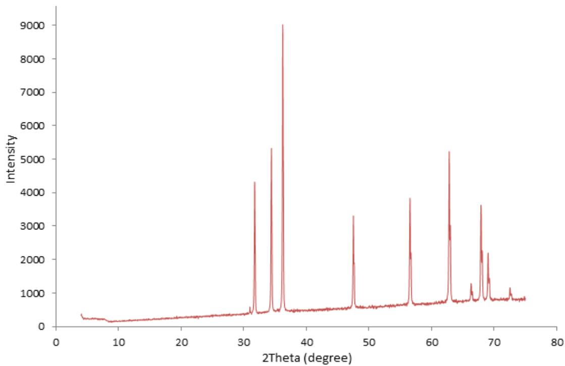
**Figure 1.** XRD pattern of the synthesized ZnO.
