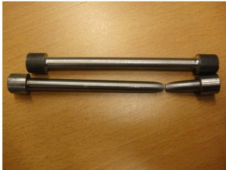
Figure 4. The tensile specimen before and after rupture.
