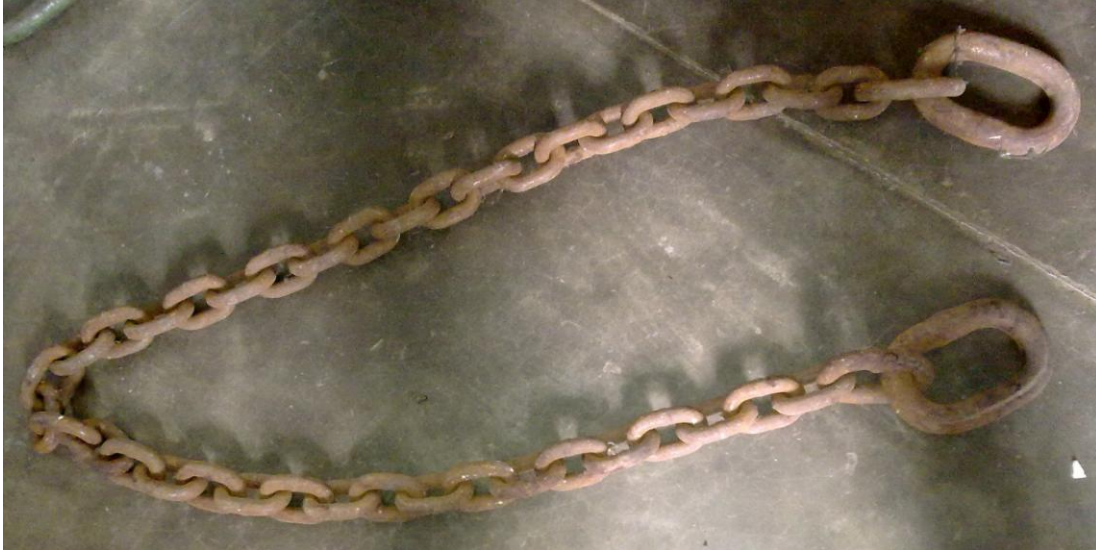
Figure 1. Bridle chain with short link, intermediate link and end link.
