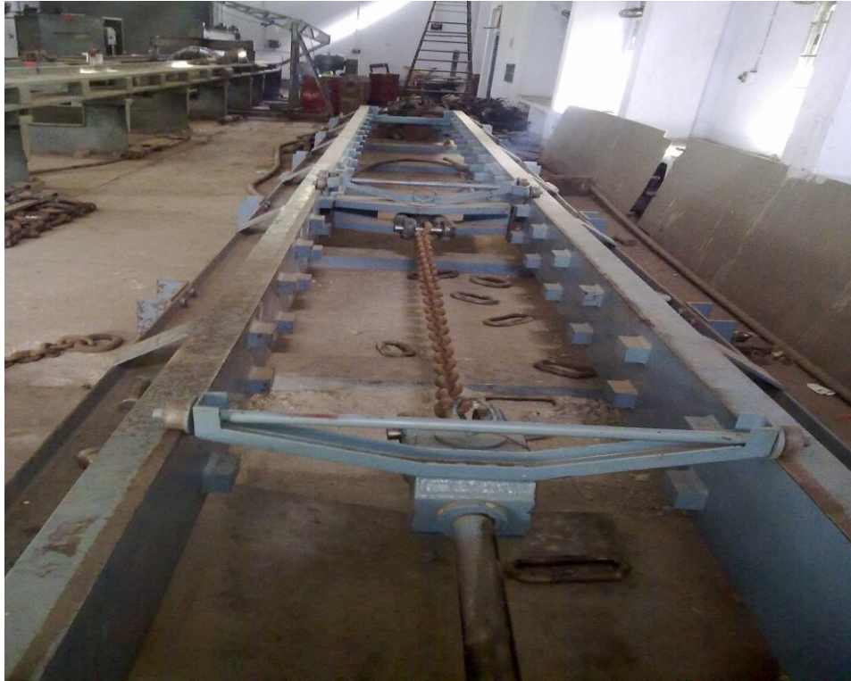
Figure 2. Static proof Load sustain in bridle chains at CIMFR laboratory in India.
