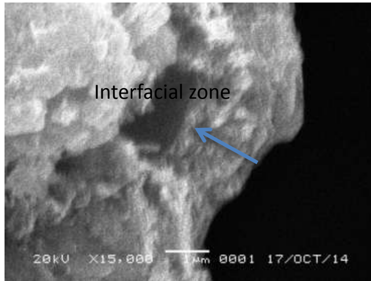
Figure 6. Microstructure of polymer modified concrete.
