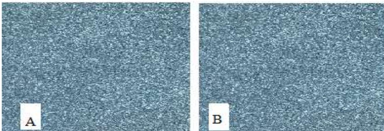
**Figure 1.** Images of RHA made using Kodak C1530 Digital Camera with 14 megapixels and 3X optical zoom. A. FRHA calcined at 700°C and in B. ORHA burnt on top of a hot metallic plate in open air.
