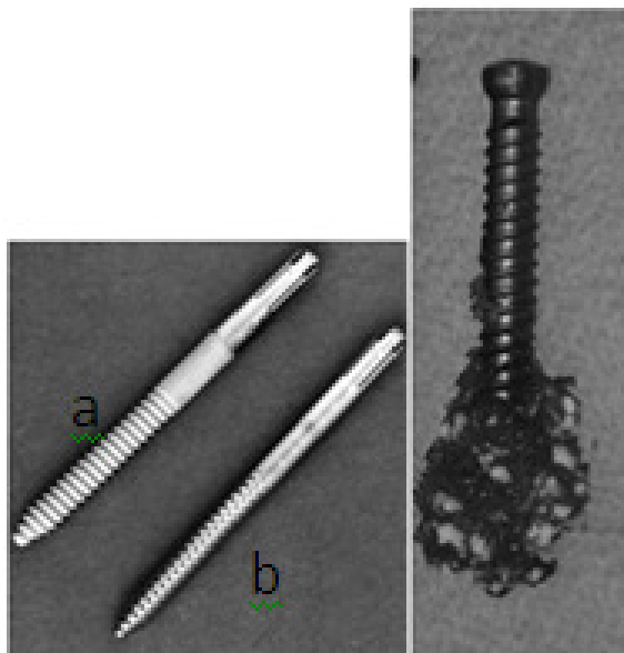
Figure 4. a) Coated and b) uncoated screws (left) and PMMA augmented screw (right) [19, 30].
