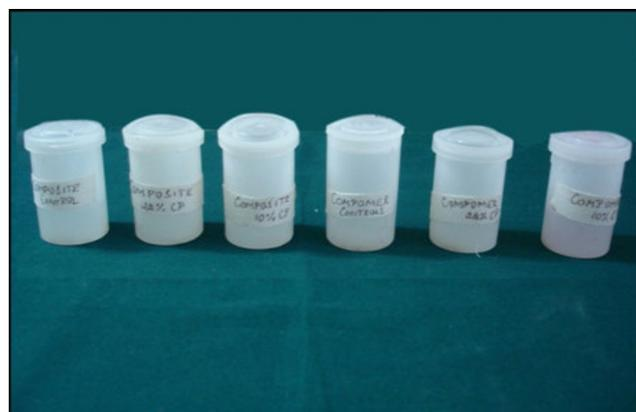
**Figure 6.** Composite and compomer pellets stored in plastic containers before microhardness evaluation.
