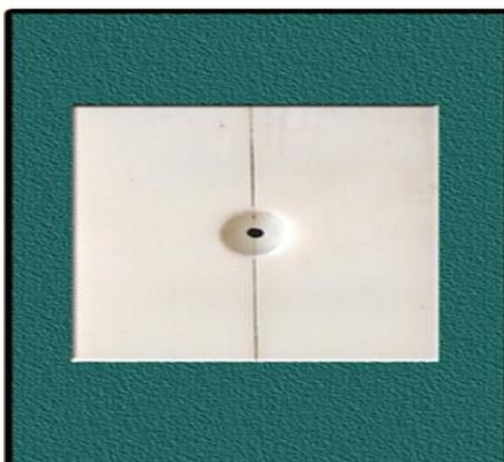
**Figure 5.** Teflon mold for preparation of shear bond strength specimens.
