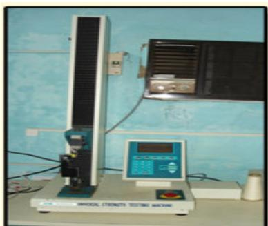
Figure 10. Universal testing machine.
