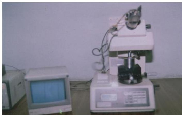
Figure 8. Microhardness testing unit and the view of an indentation.
