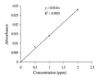
**Figure 2.** Calibration curve of standard Lead solution (Williams and Fleming, 1973).
