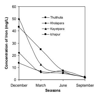
Figure 3. Seasonal variation of Iron (mg/L) in water samples at different locations of the Balu River.
