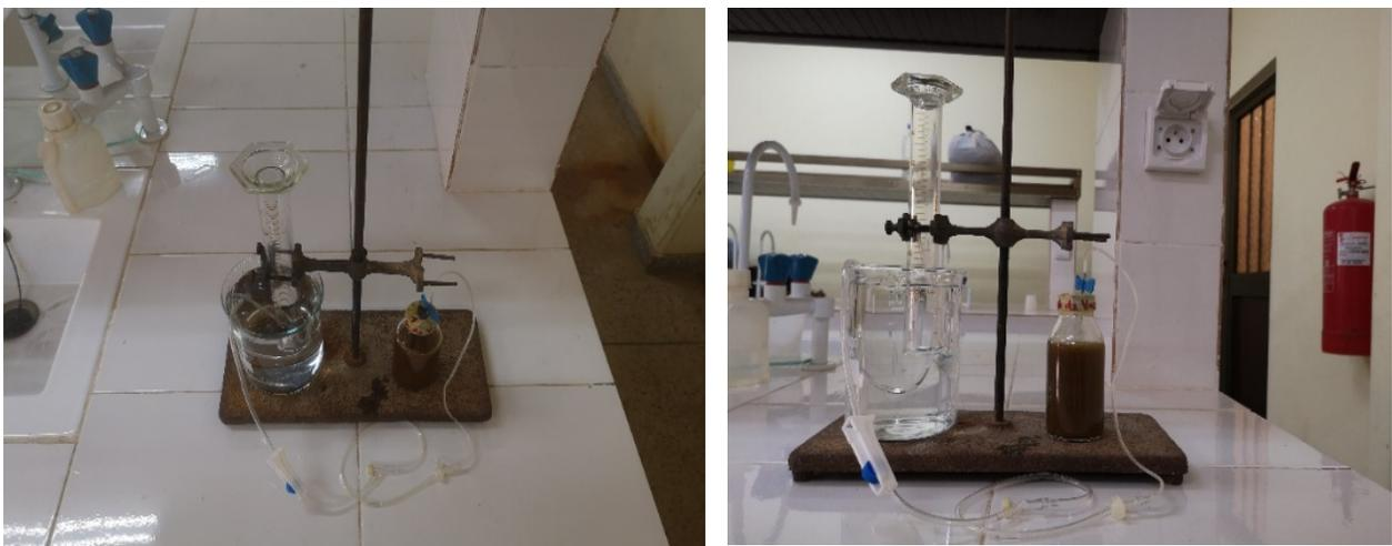
Figure 3. Device for producing the volume of biogas and methane.
