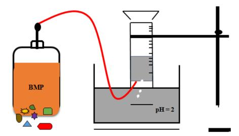
Figure 2. Device for carrying out the pretest.
