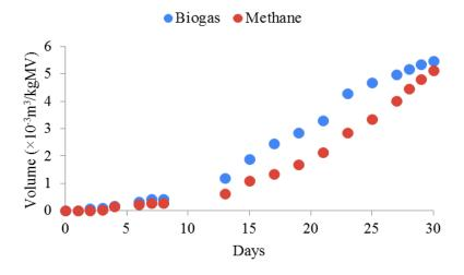
**Figure 5.** Cumulative production of biogas and methane from the inoculum (BAC5) (B).
