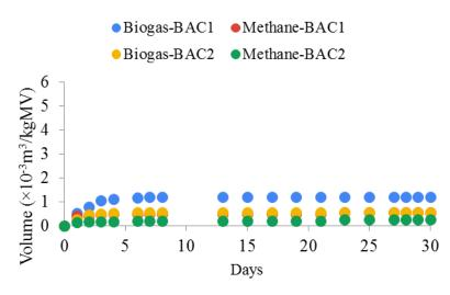
Figure 6. Cumulative production of biogas and methane from reactors by incubation.
