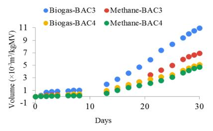
Figure 7. Cumulative production of biogas and methane from reactors by fermentation.
