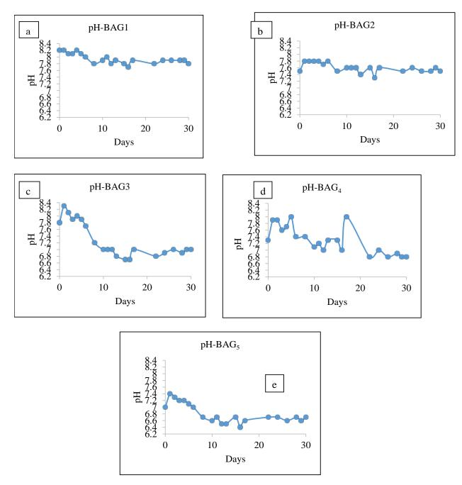
Figure 9. Daily variation in pH in the different reactors: a) D. b) S. c) DB. d) SB. e) B
