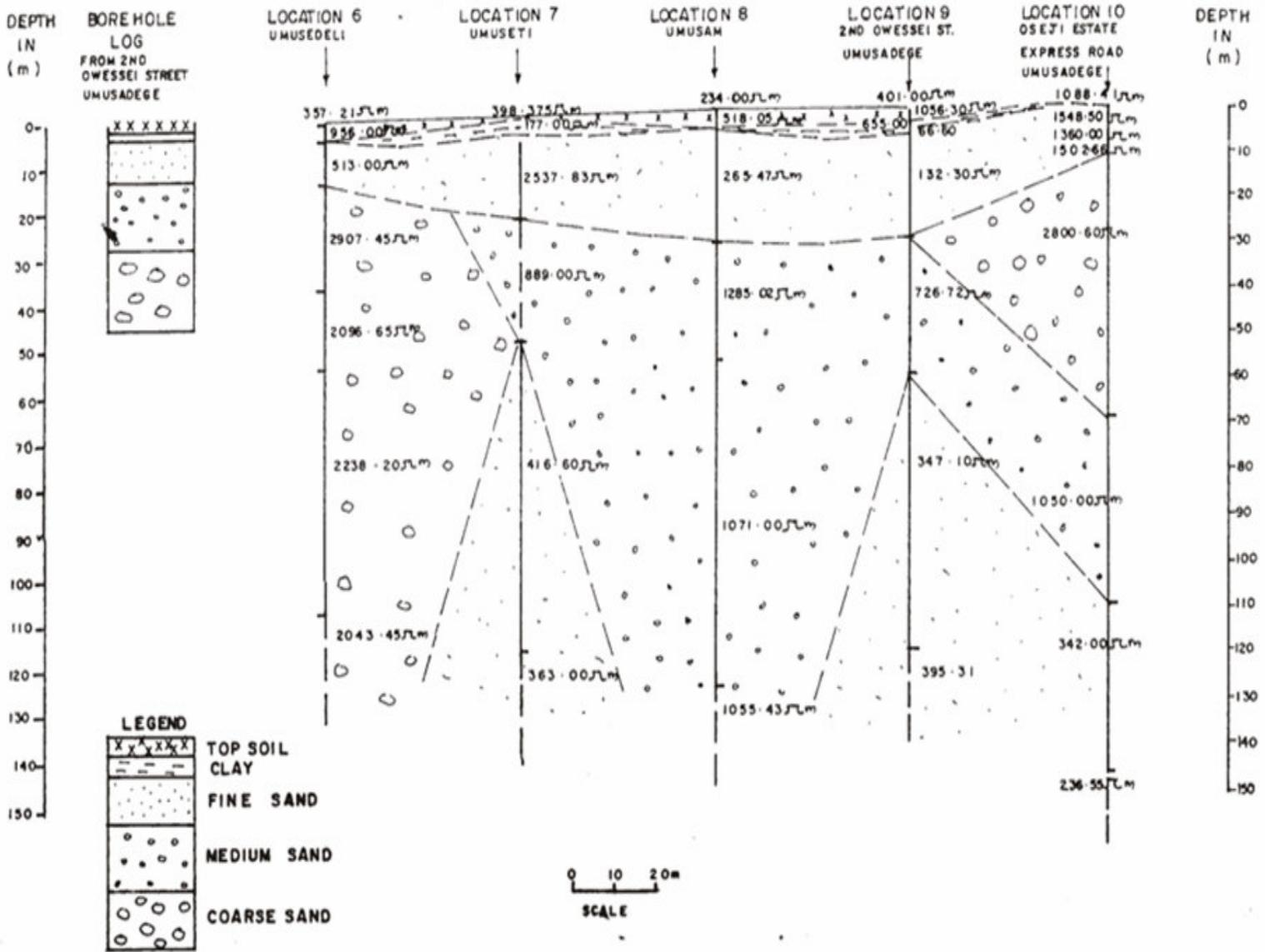
Figure 1. Geoelectric section of Utagba-Ogbe kingdom.
