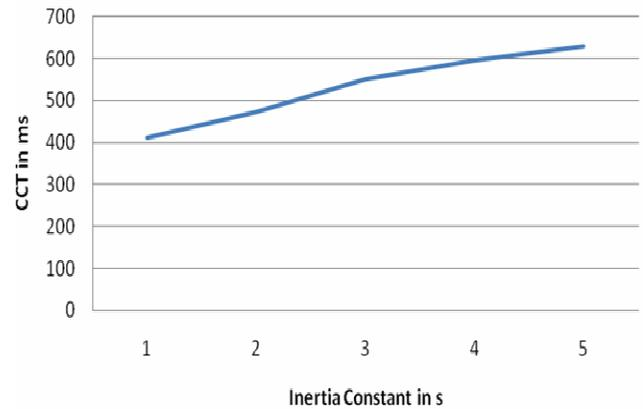
Figure 4. Relation between the inertia constant of a microturbines and CCT.
