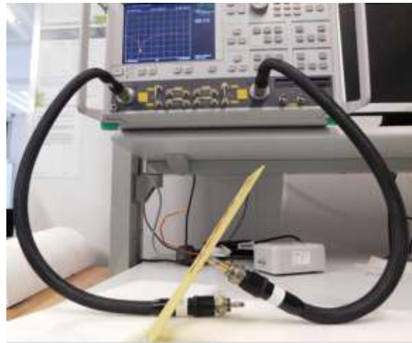
Figure 4. Measurement set up with Anritsu 37397D Vector Network Analyser.
