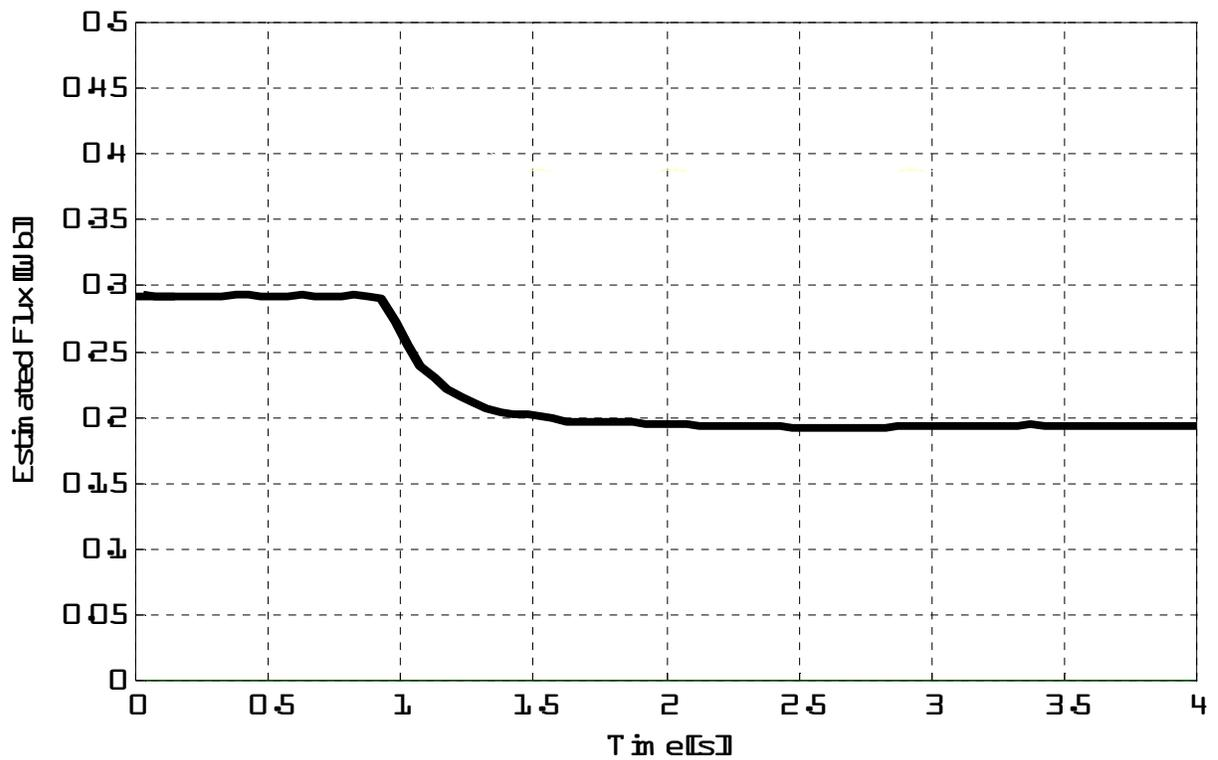
Figure 9. Experimental results for estimated of magnet flux (25% load, 200 rpm).
