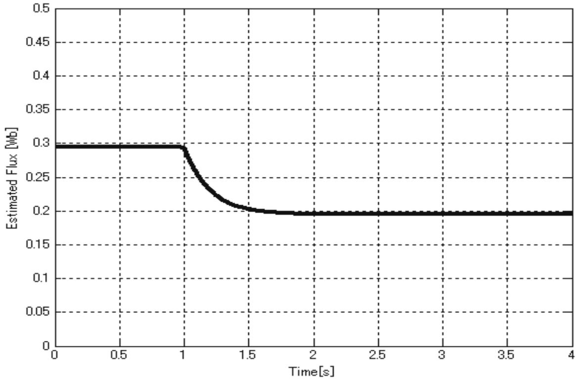
Figure 6. Simulation result for estimated for magnet flux (25% load, 200 rpm).
