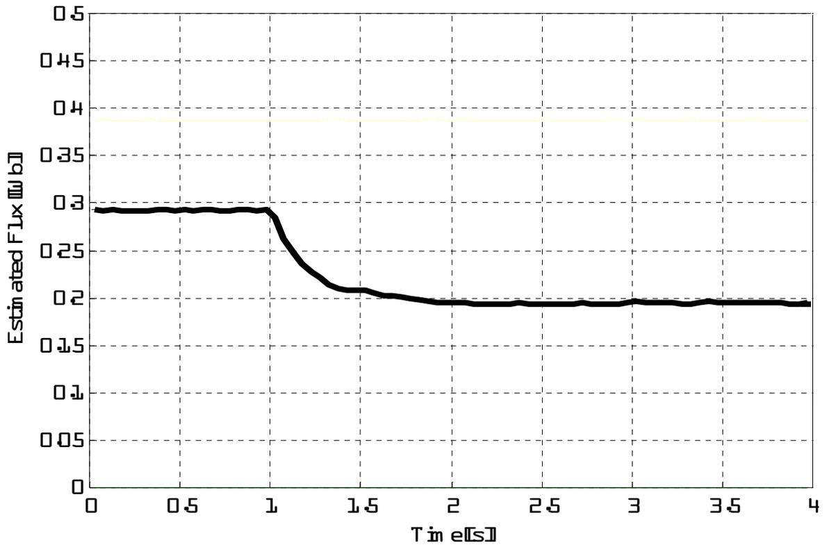
Figure 8. Experimental results for estimated of magnet flux (25% load, 20 rpm).
