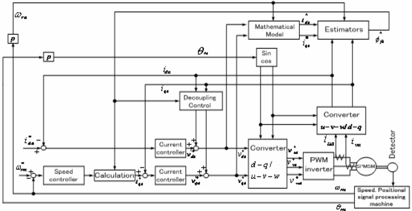
Figure 1. Block diagram of the control scheme.
