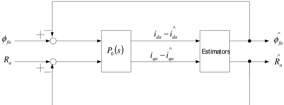
Figure 2. Construction of estimation system.
