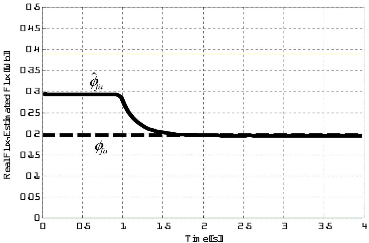
Figure 7. Experimental results for estimated of magnet flux (no-load, 20 rpm).
