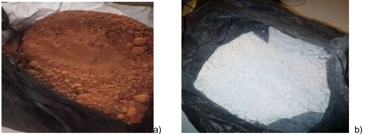
Figure 2. Partial view of a) red and b) white locally available inert dusts.
