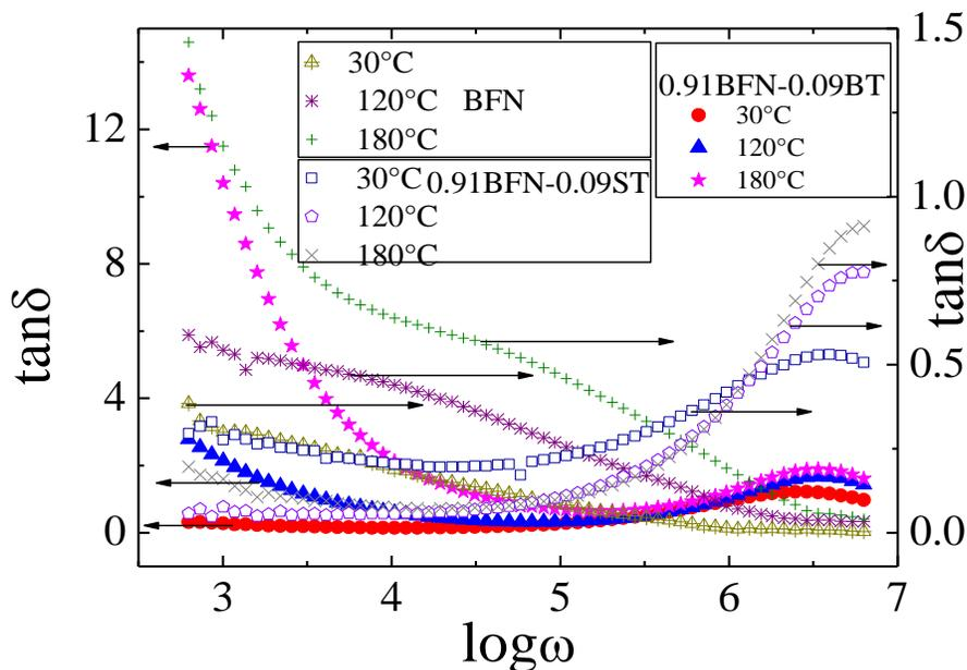
**Figure 4.** Tangent loss ( $\tan\delta$ ) of BFN, 0.91BFN-0.09BT and 0.91BFN-0.09ST, as a function of logarithmic angular frequency at various temperatures.
