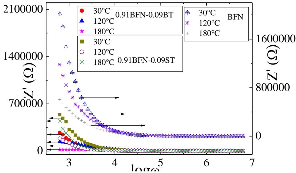
**Figure 7.**  $Z'$  of BFN, 0.91BFN-0.09BT and 0.91BFN-0.09ST, ceramics as a function of logarithmic angular frequency at various temperatures.
