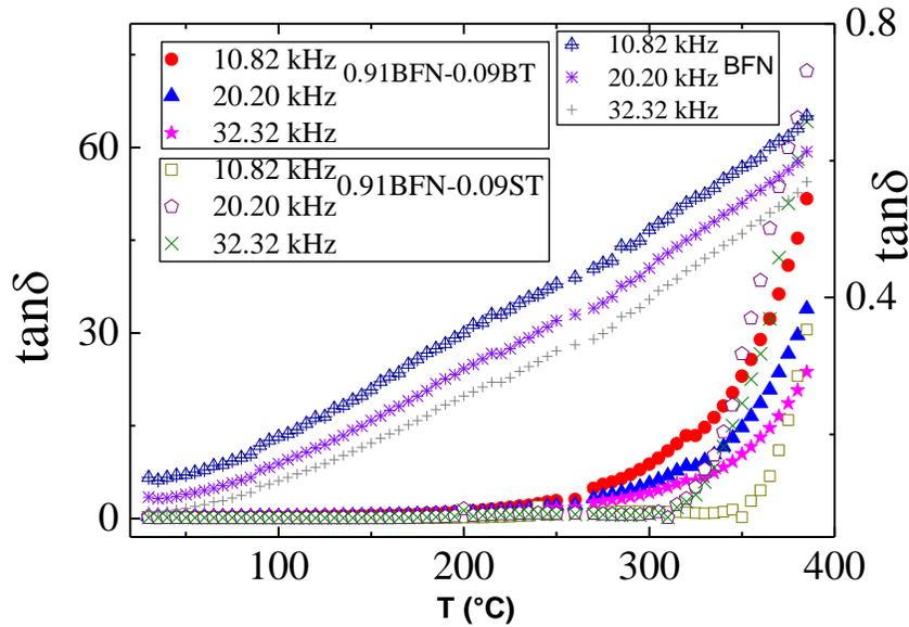
**Figure 6.** Tangent loss ( $\tan\delta$ ) of BFN, 0.91BFN-0.09BT and 0.91BFN-0.09ST, ceramics as a function of temperature at selected frequencies.
