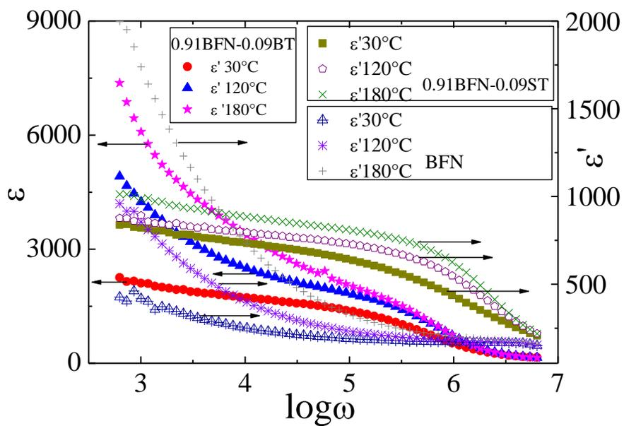
Figure 3. Logarithmic angular frequency dependence of dielectric constant ( $\epsilon'$ ) of BFN, 0.91BFN-0.09BT and 0.91BFN-0.09ST, ceramics, at various temperatures.
