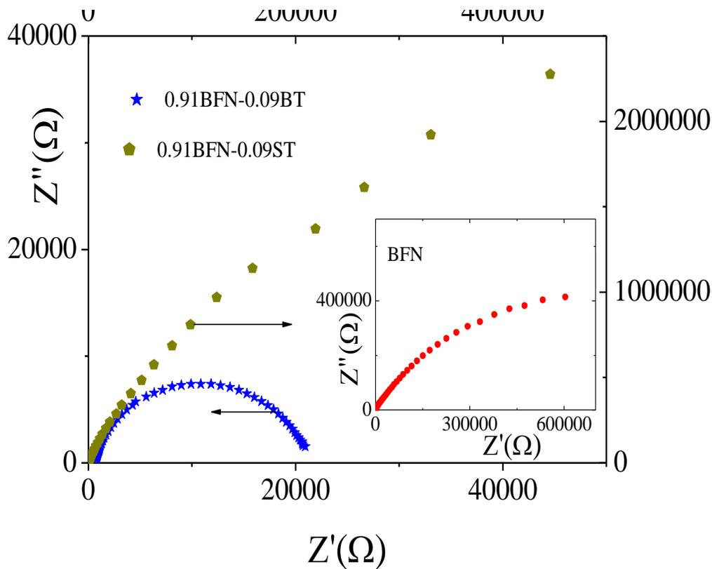
**Figure 9.** Complex plane impedance plot of BFN, 0.91BFN-0.09BT and 0.91BFN-0.09ST, ceramics, at 180°C.
