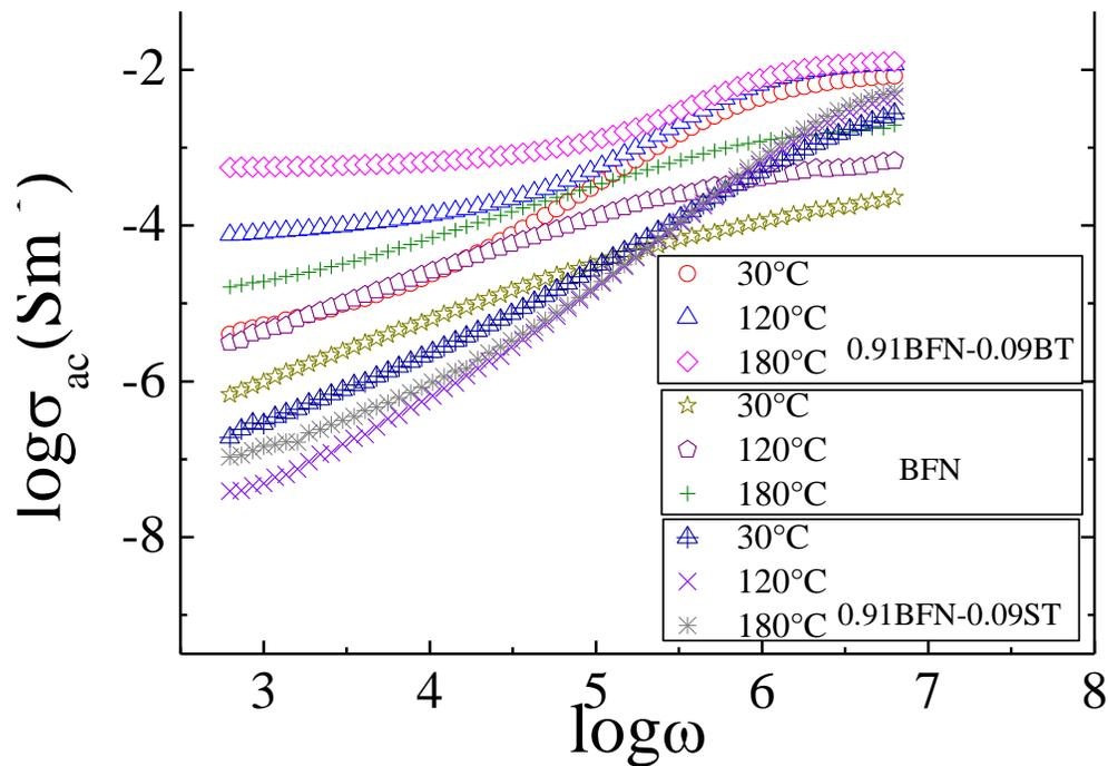
**Figure 10.** Logarithmic angular frequency dependence of ac conductivity ( $\sigma_{ac}$ ) for BFN, 0.91BFN-0.09BT and 0.91BFN-0.09ST ceramics at various temperatures.
