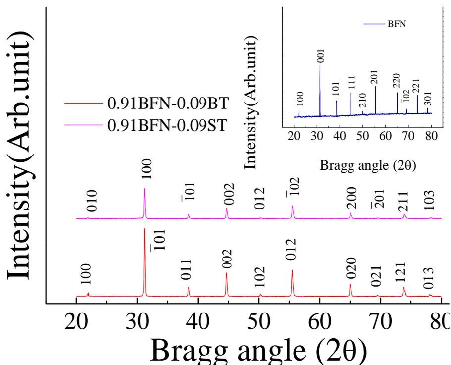
**Figure 1.** XRD patterns of BFN, 0.91BFN-0.09BT and 0.91BFN-0.09ST ceramics at room temperature.
