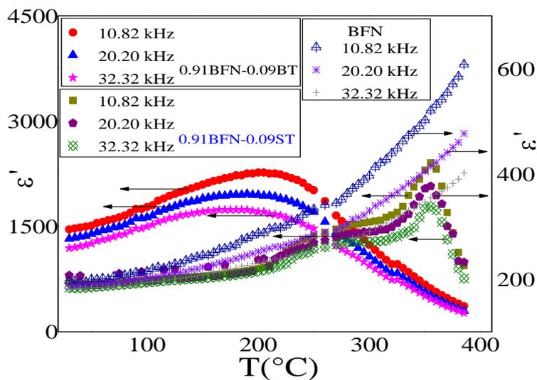
**Figure 5.** Dielectric constant ( $\epsilon'$ ) of BFN, 0.91BFN-0.09BT and 0.91BFN-0.09ST, ceramics as a function of temperature at selected frequencies.
