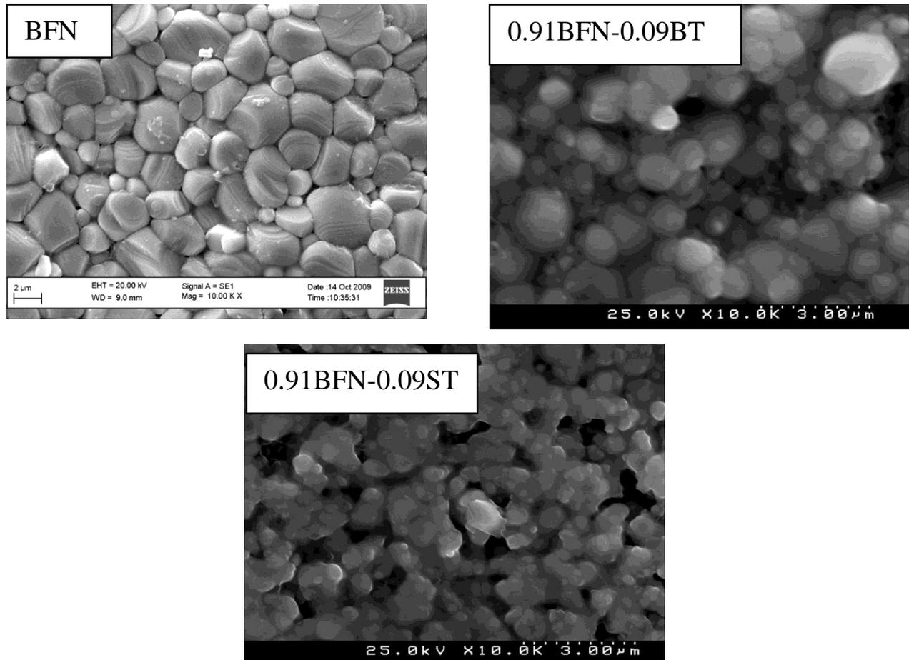
Figure 2. SEM micrographs of BFN, 0.91BFN-0.09BT and 0.91BFN-0.09ST, ceramics at room temperature.
