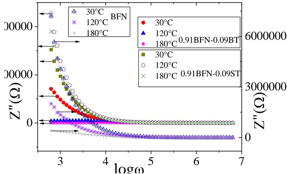
**Figure 8.**  $Z''$  of BFN, 0.91BFN-0.09BT and 0.91BFN-0.09ST, ceramics as a function of logarithmic angular frequency at various temperatures.
