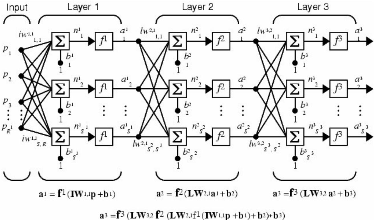
Figure 3. Three layer feed forward artificial neural network.
