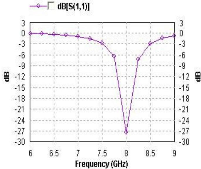
Figure 2. The return loss ( $S_{11}$ ) in dB verses resonating frequency of microstrip antenna.
