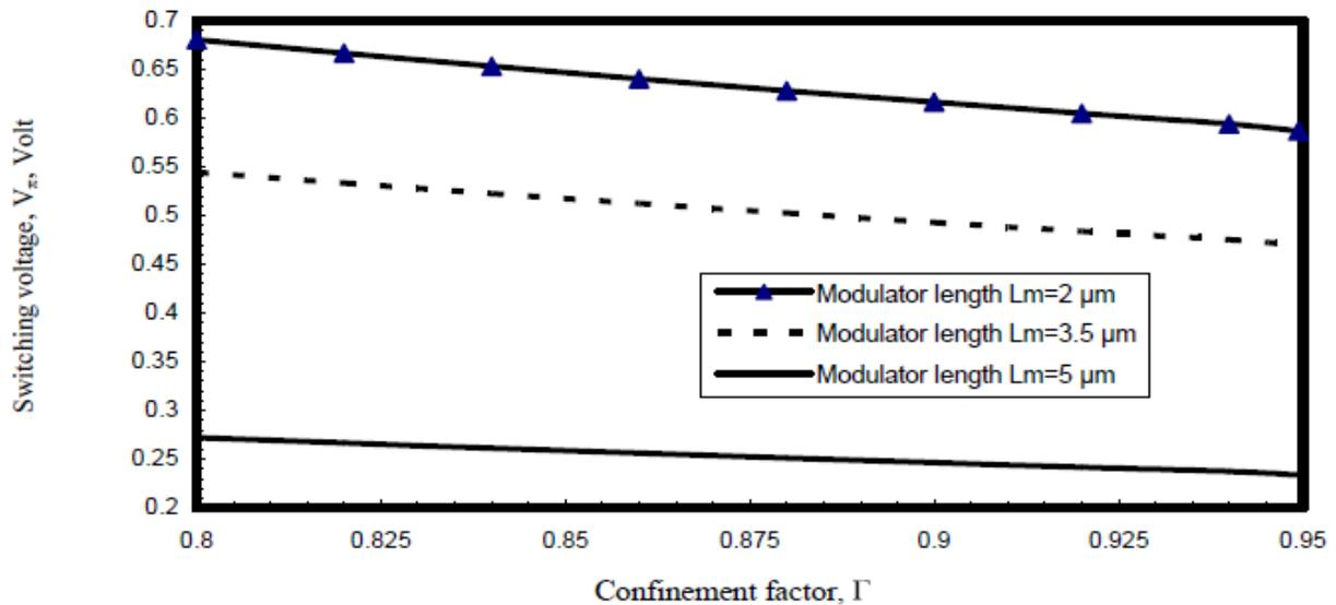
**Figure 1.** Variations of switching voltage versus confinement factor at the assumed set of parameters.
