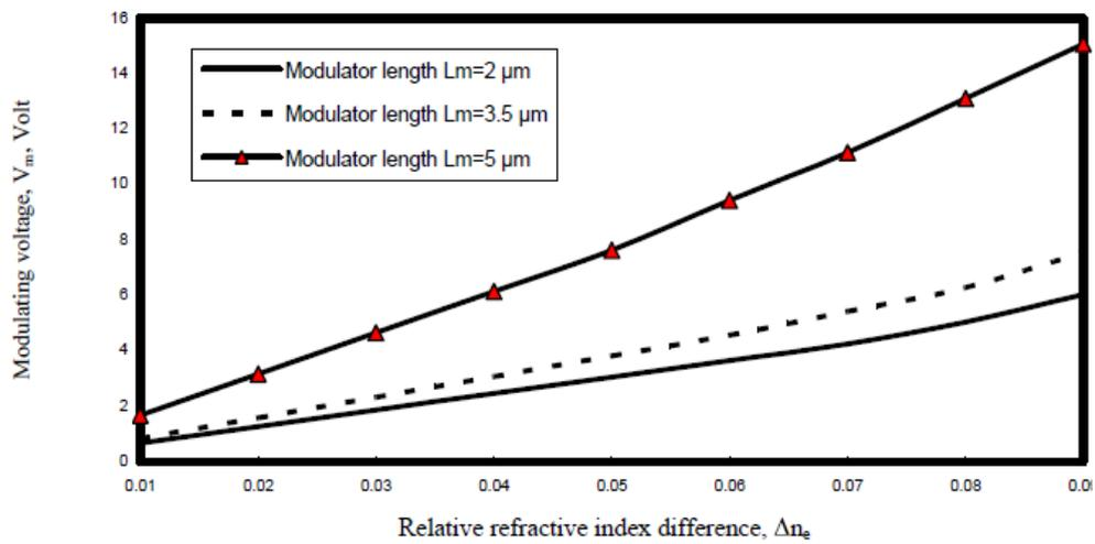
Table 4. Variations of modulating voltage against relative refractive index difference at the assumed set of parameters.
