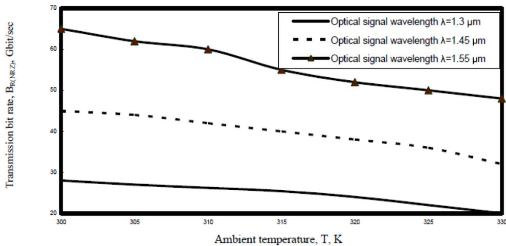
**Figure 13.** Variations of transmission bit rate versus ambient temperature at the assumed set of parameters.
