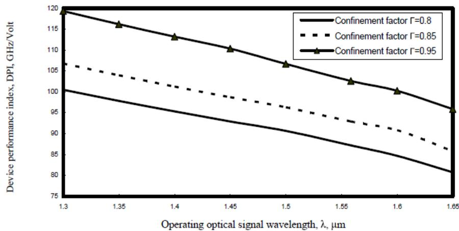
**Figure 7.** Variations of device performance index optical signal wavelength at the assumed set of parameters.
