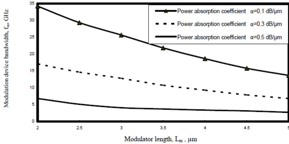
**Figure 5.** Variations of modulation bandwidth against modulator length at the assumed set of parameters.
