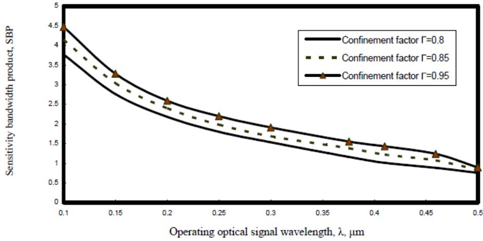
**Figure 8.** Variations of sensitivity bandwidth product against optical signal wavelength at the assumed set of parameters.
