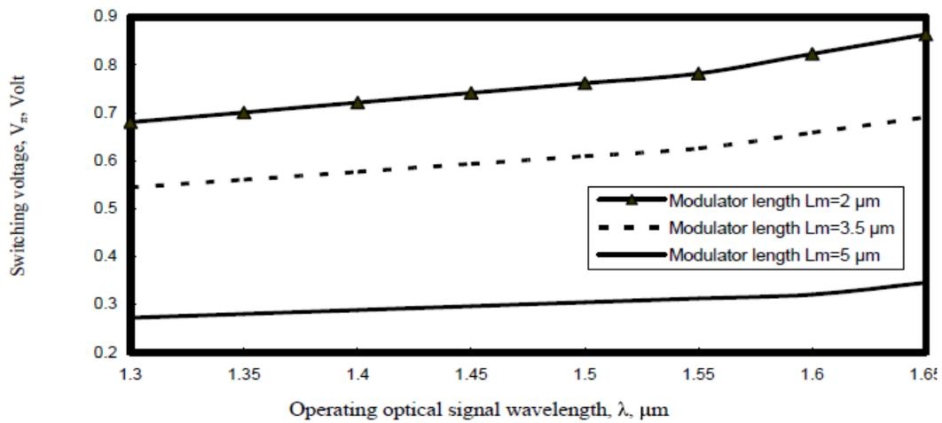
Table 3. Variations of switching voltage versus signal wavelength at the assumed set of parameters.
