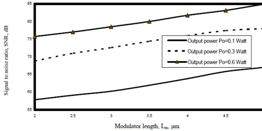
**Figure 9.** Variations of signal to noise ratio against modulator length at the assumed set of parameters.
