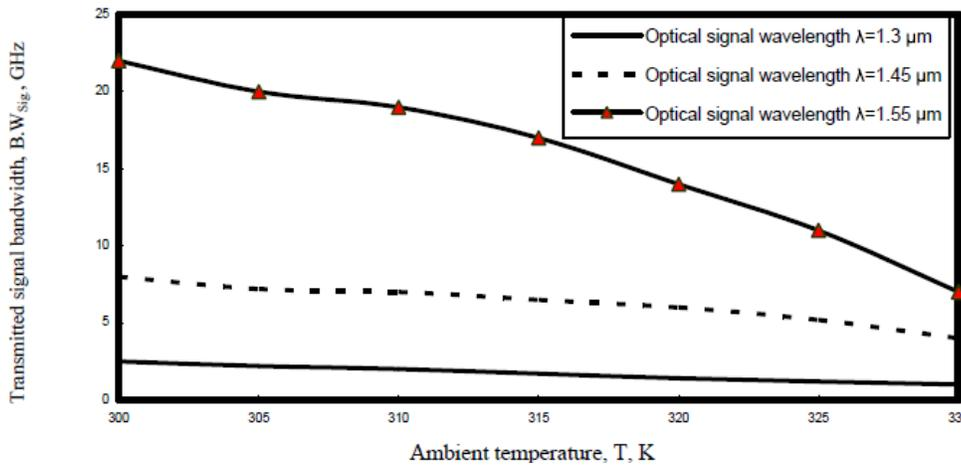
**Figure 12.** Variations of transmitted signal bandwidth versus ambient temperature at the assumed set of parameters.
