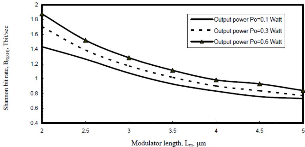
**Figure 10.** Variations of Shannon transmission bit rate against modulator length at the assumed set of parameters.
