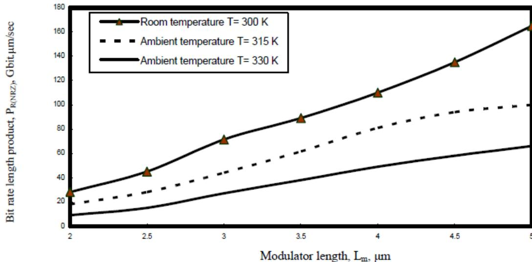
**Figure 14.** Variations of transmission bit rate length product against modulator length at the assumed set of parameters.
