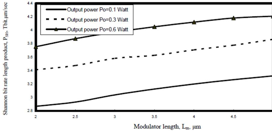
**Figure 11.** Variations of Shannon bit rate length product against modulator length at the assumed set of parameters.
