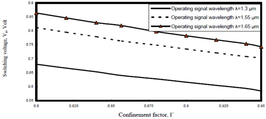
Figure 2. Variations of switching voltage versus confinement factor at the assumed set of parameters.
