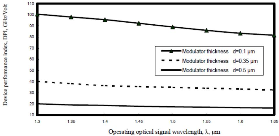
**Figure 6.** Variations of device performance index against optical signal wavelength at the assumed set of parameters.
