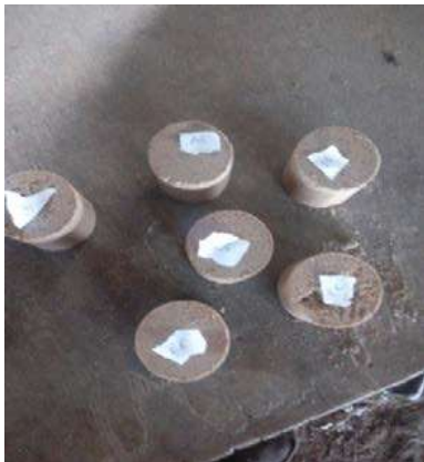
Figure 5. Sand test samples for permeability test.
