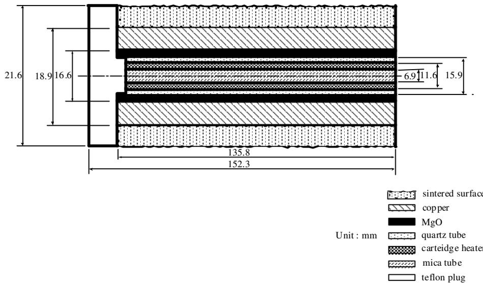
Figure 2. Schematic of test section.
