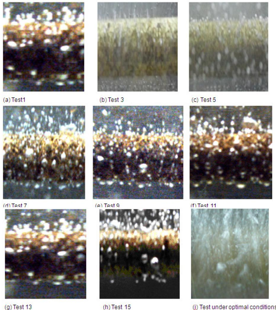
**Figure 5.** Photos of bubble formation in nucleate boiling under different test conditions, as shown in Table 1 and in the test under the optimal conditions.
