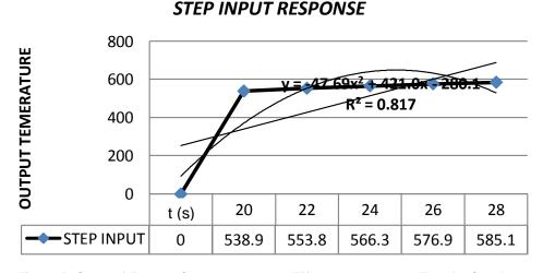
**Figure 5.** Graph of Furnace Output temperature T(t) responses versus Time for Step Input Response using polynomial and linear trend.
