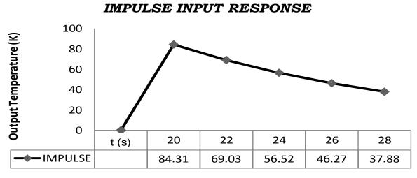
Figure 4. Graph of Furnace Output temperature T(t) responses versus Time for Impulse Input Response.
