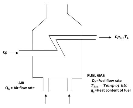
Figure 1. A preheating furnace.
