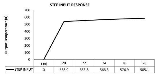
Figure 2. Graph of Furnace Output temperature T(t) responses versus Time for Step Input Response.
