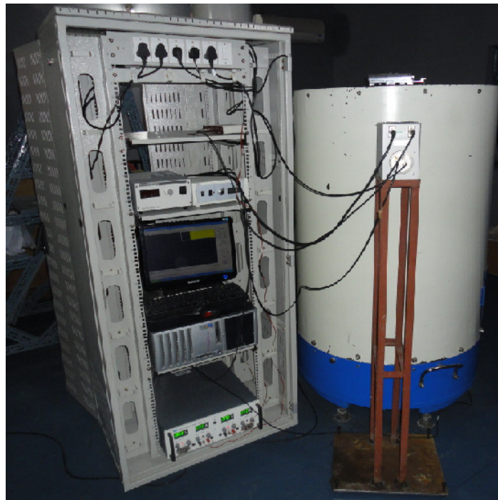
Figure 8. Assembled LIDAR receiver telescope with detection optics and electronics.
