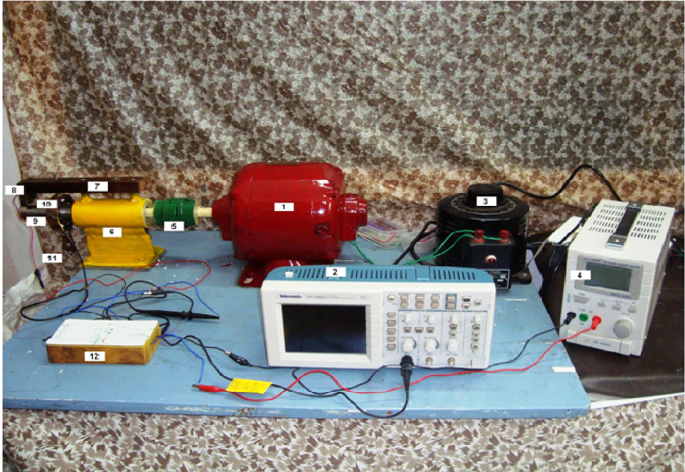
Figure 2. Photograph of rolling element bearing test rig; 1, DC motor; 2, Storage oscilloscope; 3, Variable AC transformer; 4, Regulated DC supply; 5, Flexible coupling; 6, Supporting shaft assembly; 7, Wooden cantilever; 8, Carbon brush assembly; 9, Stainless steel sleeve; 10, Copper sleeve over test bearing; 11, Hook for radial loads; 12, Electrical circuit.
