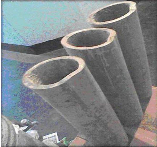
Figure 1. Prepared bamboo sample for compression test.
