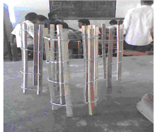
Figure 4. Preparation of bamboo reinforcement case with tie bar.
