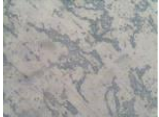
Plate 3. Photomicrograph of 1.0 mm mild steel immersed in cassava fluid (x400; Etched in 2% Nital and 98% Ethly alcohol).
