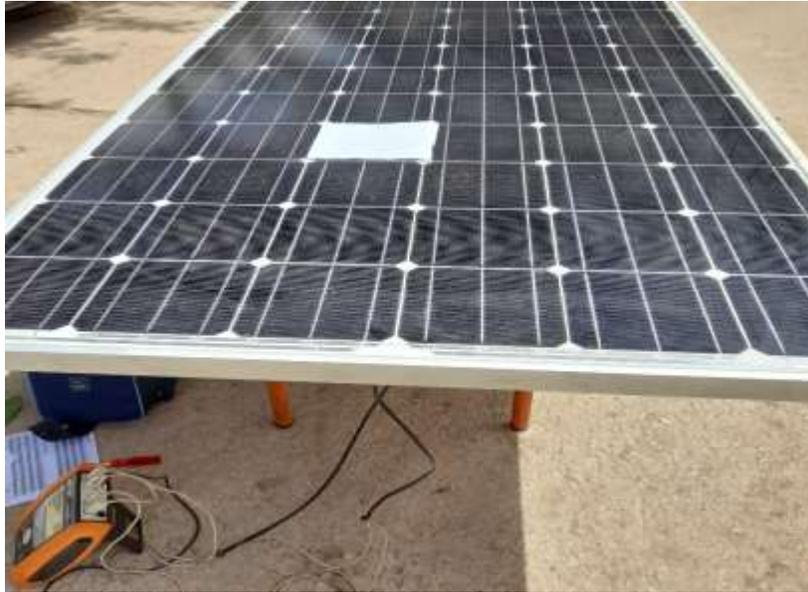
**Figure 1.** Mono module under test in partial shade.
