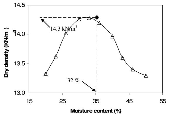
Figure 2. Plot of moisture content versus dry density.
