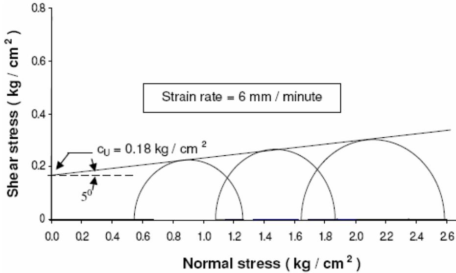
Figure 5. Mohr circle diagram for U.U. triaxial test.
