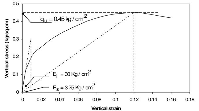
Figure 3. Unconfined compression test results.
