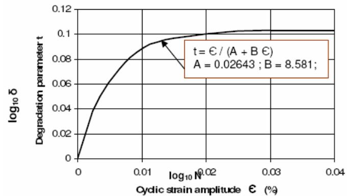
**Figure 10.** A plot of degradation parameter versus cyclic strain amplitude.
