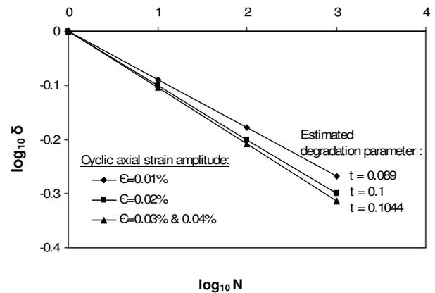
**Figure 9.** A plot of degradation index versus no. of cycles in log-log scale.
