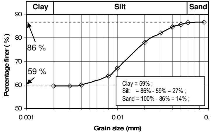
Figure 1. Grain size distribution curve.
