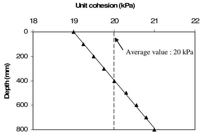
Figure 7. Variation of unit cohesion with depth.
