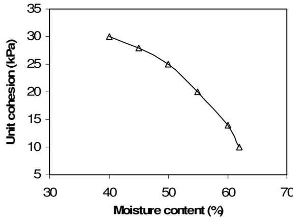
Figure 8. Variation of unit cohesion with moisture content.
