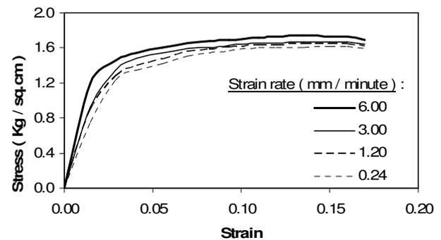
Figure 4. Stress-strain curves obtained from U.U. triaxial tests.
