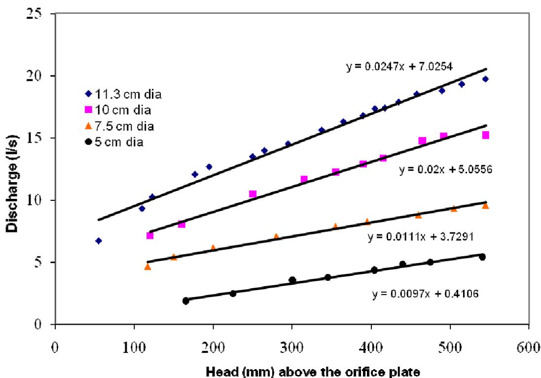
**Figure 3.** Rating curve for orifice bucket.
