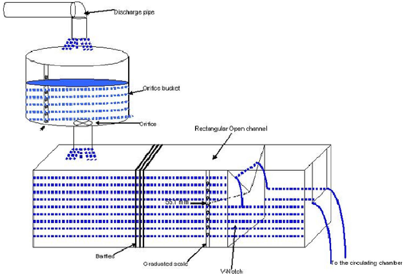
Figure 2. Schematic sketch of the calibration circuit.
