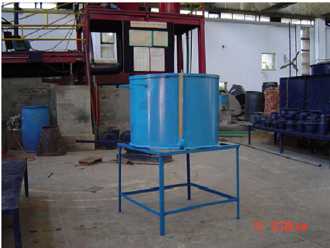
**Plate 2.** Fabricated orifice bucket (Side view).
