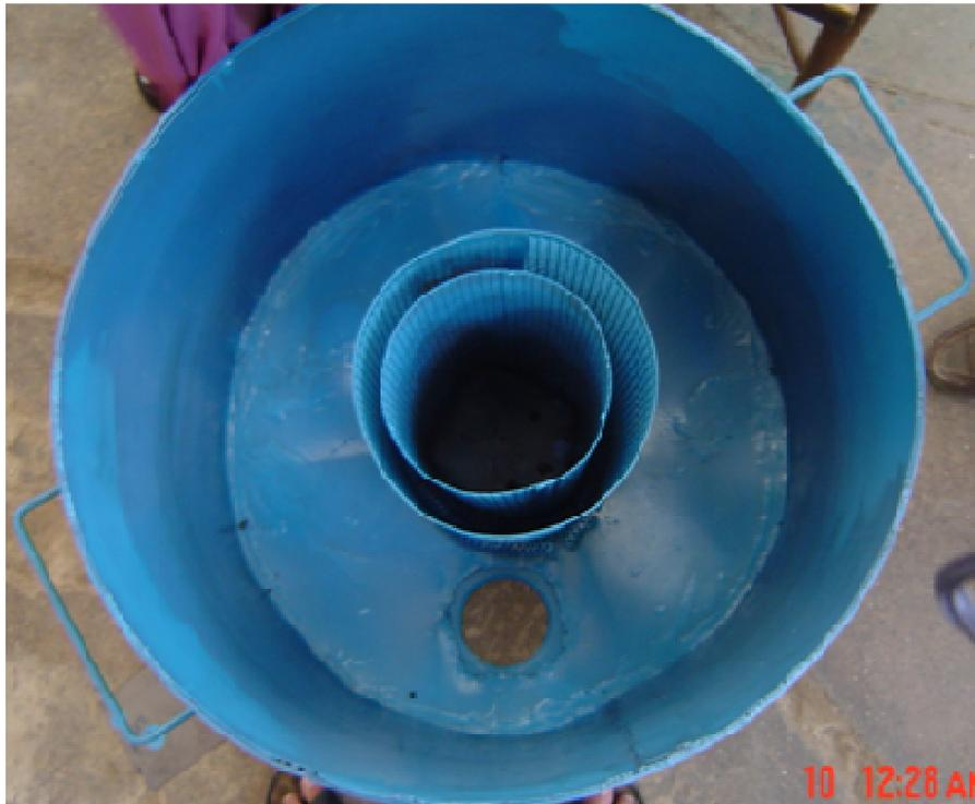
**Plate 1.** Fabricated orifice bucket (Top view).
