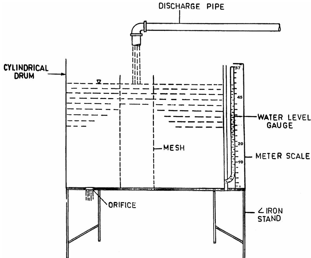
Figure 1. Schematic sketch of orifice bucket (not to scale).
