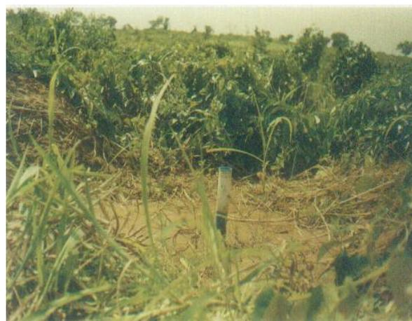
Figure 3. Installed Peizometer.
